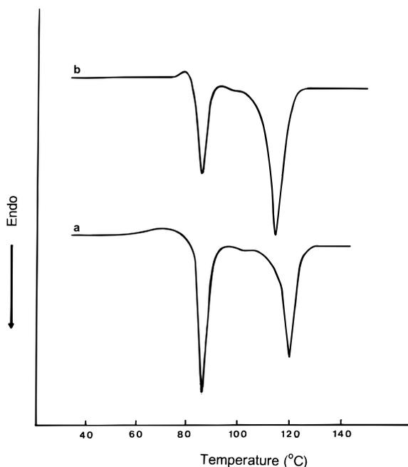
**Figure 1.** DSC traces of (a) 1:1 and (b) 2:1 mixtures of adenine-barbituric derivatives.
