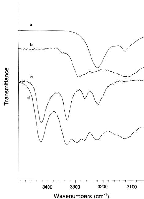
**Figure 2.** FT-IR spectra of (a) barbituric and (b) adenine derivatives as well as of their (c) 1:1 and (d) 1:2 mixtures.
