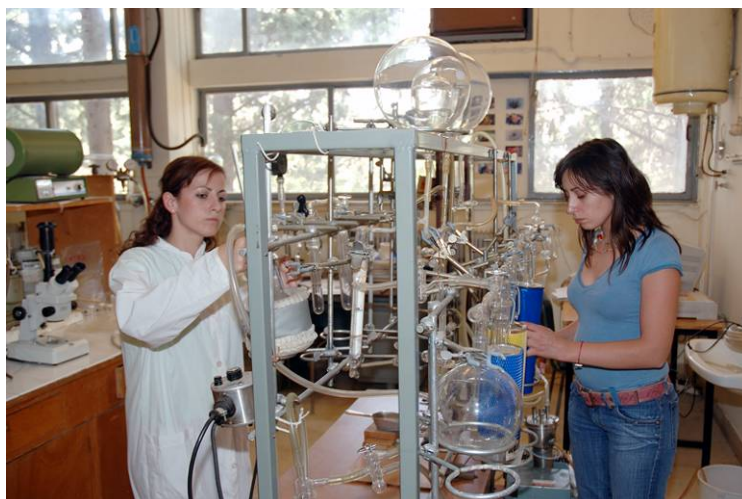
Synthesis of benzene samples for Radiocarbon dating.
